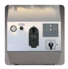
Simple and intuitive control panel, quick-coupling steam gun, main ON/OFF switch with lamp, boiler resistance activation lamp, steam flow rate regulator, steam ready indicator lamp, steam pressure gauge. Steam gun with integrated steam/detergent function activation key and quick coupling of accessories. Boiler no water safety stop sensor. No water and water tank full lamp. Water pump activation lamp.
