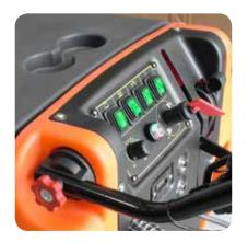
User friendly analogic control panel. Control lever for brush operation and detergent water outflow. ON/OFF and battery cutout key switch, brush and vacuum motor switch, detergent dosing knob (optional), Thermal circuit breaker to protect vacuum and brush motor, battery level indicator, hour meter (optional).
