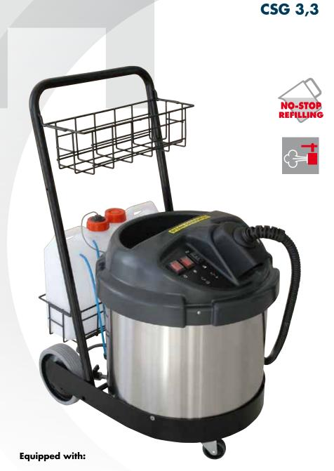
• Satured steam at 9 bar at a temperature of 175°C • Steam gun with low tension control • S/S body AISI 304 • Boiler 3,3 kW S/S AISI 304. Thickness 25/10 • Low level water lamp indicator • Device for using chemicals and detergents mixed with steam • Heating and activation time required: 7 min. • Steam regulation • Discharge valve • Pressure gauge • The boiler can be refilled from the tank provided (continuous duty) • Wheels suitable for food and processing areas • Storage basket
